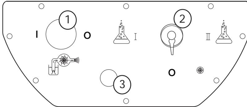
**Solution Pump Switch (1):** turns the solution pump on/off
